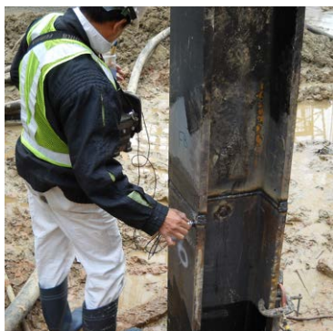
Photo HU1.7 – Test of Weld
