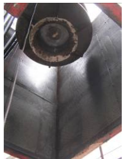
Figure H7.6(b) – Noise Muffler Enclosing Hydraulic Hammer during Percussive Piling Work
