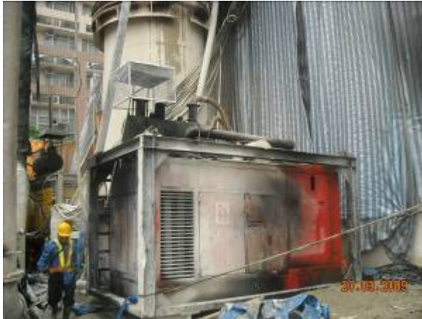
Figure H7.7 – Exhaust Purifier for Diesel Power Pack of Reverse Circulation Drill
