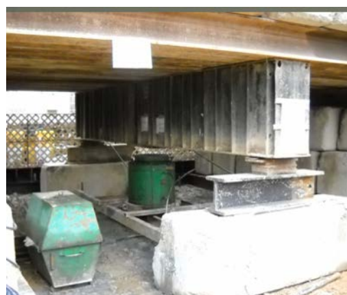
Photo HU1.14 – Static Loading Test – Close-up of Load Cell on Top of Pile
