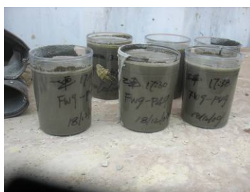
Photo HU5.8 – Initial Setting Time Test for Grout
