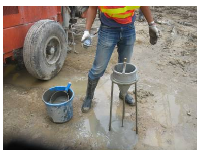
Photo HU5.7 – Flow Cone Test for Grout
