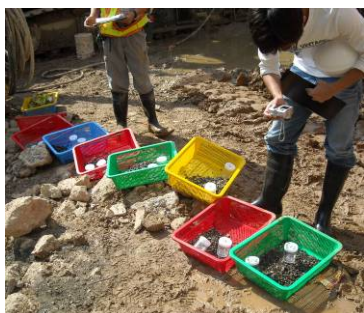
Photo HU3.10 – Obtaining Rock Sample after Completion of Drilling Operation
