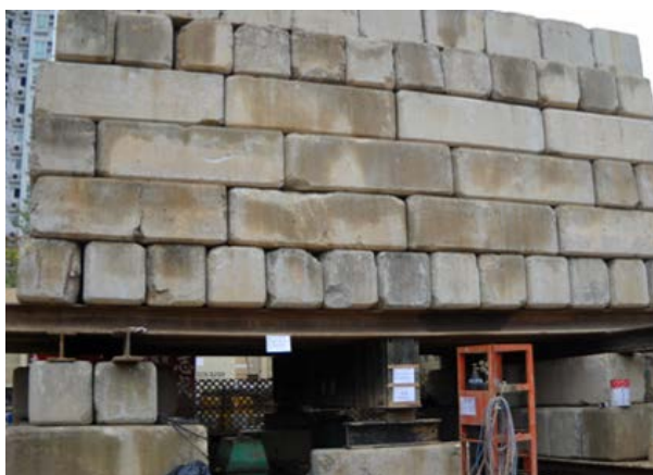
Photo HU1.13 – Static Loading Test – Set-up with Kentledge
