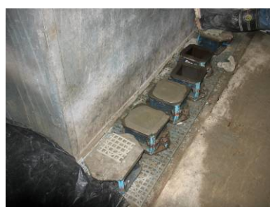
Photo HU5.9 – Grout Cube Compression Test
