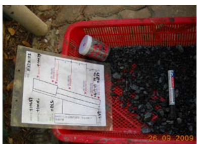
Photo HU4.6 – Collecting Rock Sample at Founding Level
