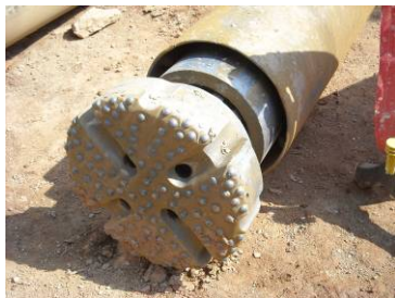
Photo HU3.4 – ODEX Drilling Bit
