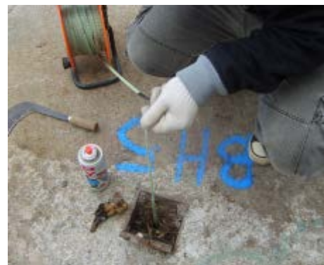
Figure H7.4(e) – Piezometer (for Checking Ground Water Level)
