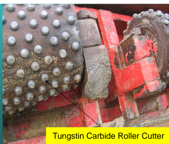
Photo HU2.5 – Excavation of rock or similar hard material using Reverse Circulation Drilling Rig for Formation of the Rock Socket.
