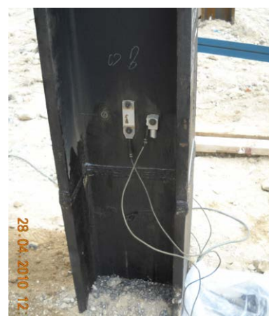
Photo HU1.9 – Installing Transducers on Pile for the PDA Test
