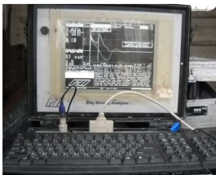
Photo HU1.10 – Pile Driving Analyzer Test Data Displayed on Screen
