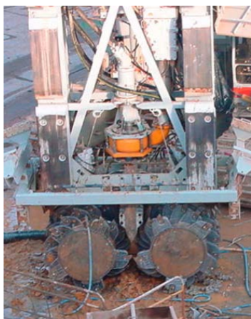
Photo HU6.4 – Cutter at the bottom of The Hydromill Machine
