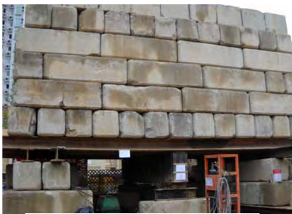
Photo HR1.12(a) – Static Loading Test – Set-up with Kentledge
