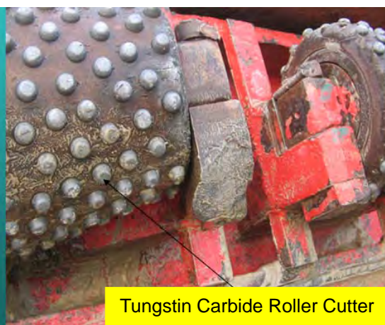
Photo HR2.5 – Excavation of rock or similar hard material using Reverse Circulation Drilling Rig for Formation of the Rock Socket.
