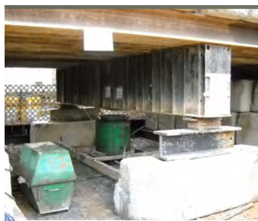
Photo HR1.12(b) – Static Loading Test – Close-up of Load Cell on Top of Pile
