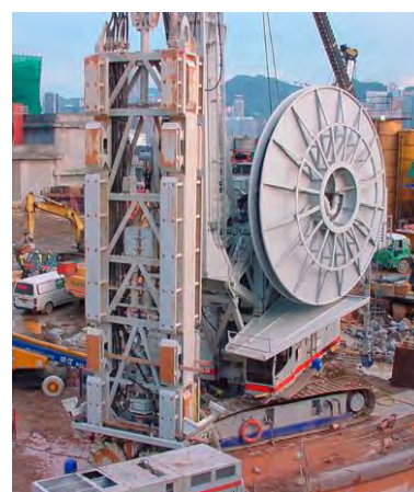
Photo HR6.3 – The Hydromill Machine for Trench Excavation
