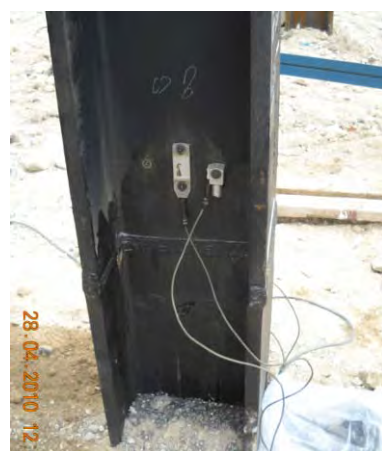
Photo HR1.9 – Installing Transducers on Pile for the PDA Test
