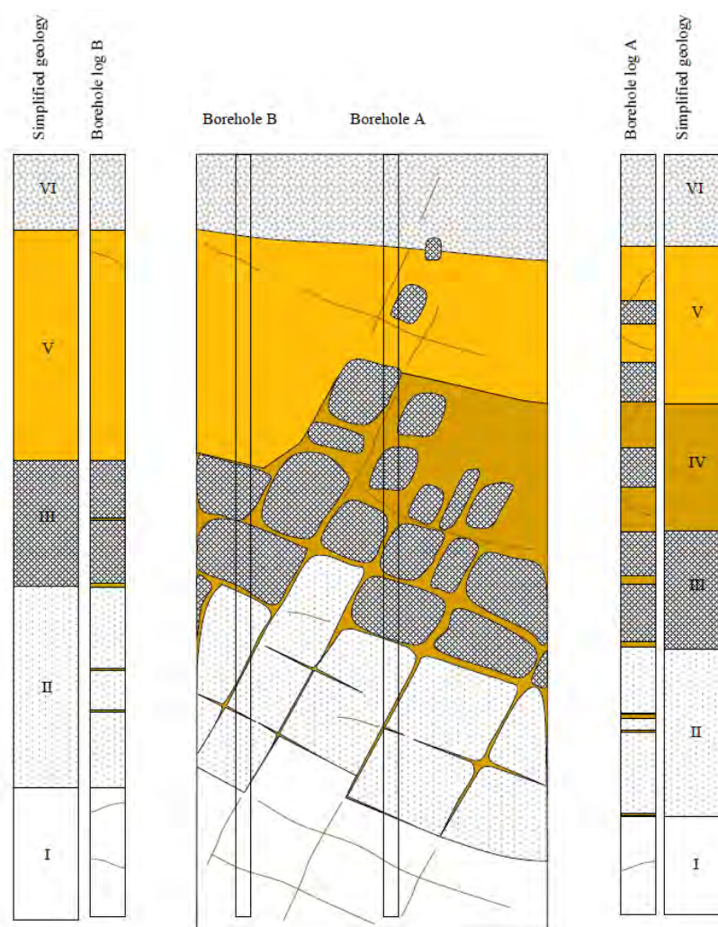
Note : Refer to Geoguide 3 (GCO, 1988) for classification of rock decomposition Grade I to VI Figure HA-1 – Representation of a Corestone-bearing Rock Mass (Malone, 1990)
