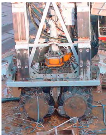
Photo HR6.4 – Cutter at the bottom of The Hydromill Machine
